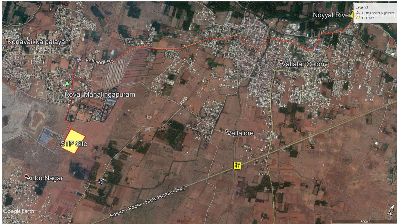
Figure 5: Sewage Treatment Plant and Alignment of Outfall Sewer
